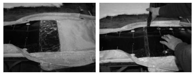
Figure 10 – Position PFA adhesive film
