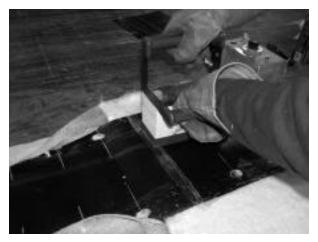
Figure 13 – Position iron and press firmly.
