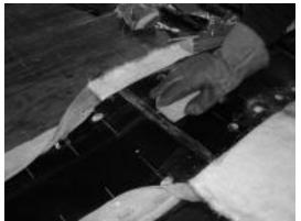
Figure 14 – Press Splice with a wooden block.
