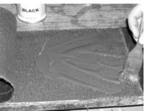
Figure 21 – Evenly spread cold splice cement.
